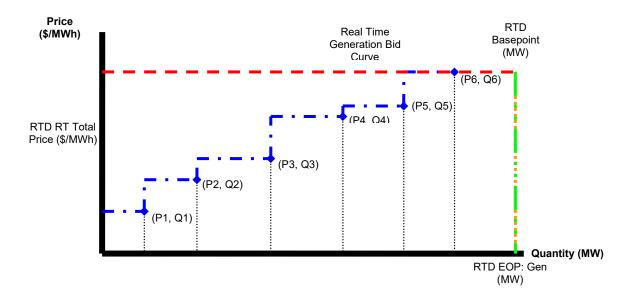
Similarly, if the RTD interval LBMP intersects the given Generation Bid block on a horizontal line and the Generator was Base Pointed within the same Bid block, the Generator's EOP is equal to its RTD Base Point.
